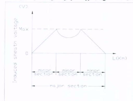
Variation of sheath voltage to earth on a Cross-bonded system
